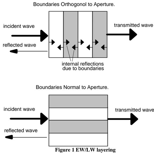
The change in polarisation of the microwave fields due to EW/LW layering has given rise to many systems proposed for the measurement of grain angle. One such system was developed by [1] which involved a rotating antenna that used the angle of the antenna and a maximum in the received signal to determine the grain angle of lumber.
